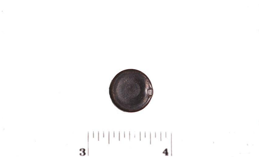
Figure 1. Firing pin impression made by a Ballard rifle.
