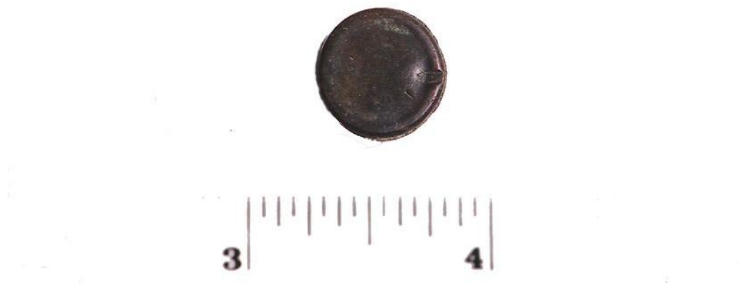
Figure 1. Firing pin impression from a Smith and Wesson Firearm.
