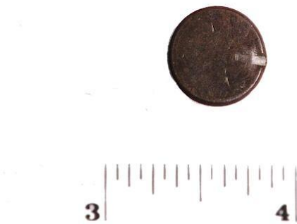
Figure 2. Firing pin impression made by a Remington Firearm.
