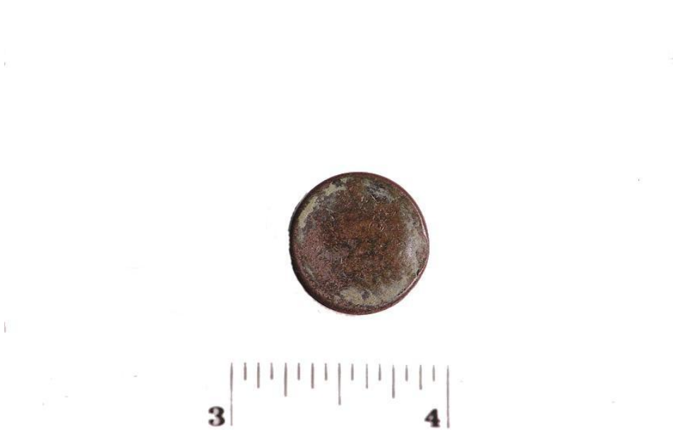
Figure 2. Note the half-moon firing pin impression on the Spencer Casing.
