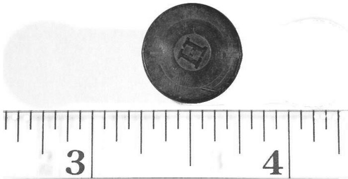
Figure 2: “Henry” Headstamp and firing pin markings on a cartridge casing fired from a Model 1866 Winchester or Henry rifle.
